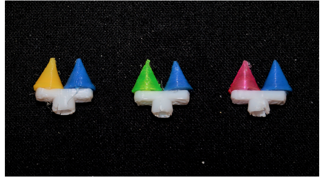
Figure 7: The three different markers used by ClipWidgets. The yellow marker is used for buttons, the green marker is used for dials and the pink marker is used for sliders. This color mapping was chosen arbitrarily
